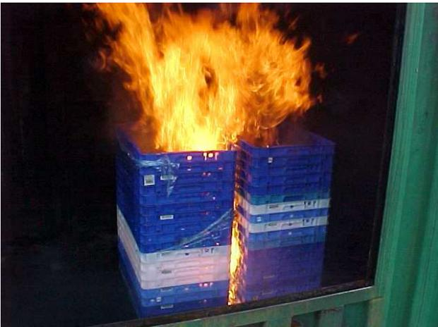
**Test 3:** Four half height stacks were formed into a square, ignited at their centre, and allowed to burn until flames were over 1 m above the top of the stacks. The foam water supply was initiated and extinguishment was again achieved after two minutes.
